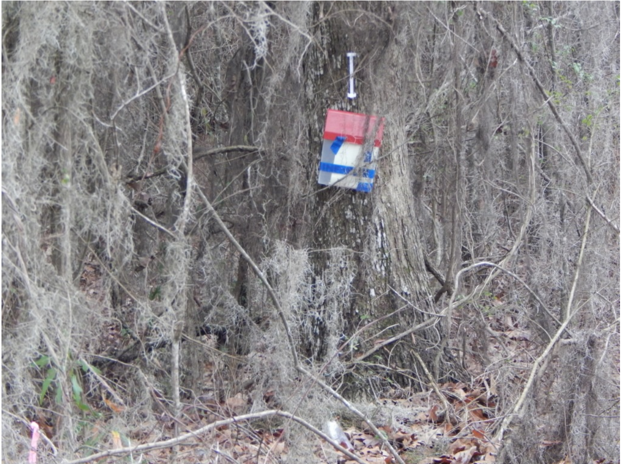
Improper Rain Gauge Placement 12.23.2013
