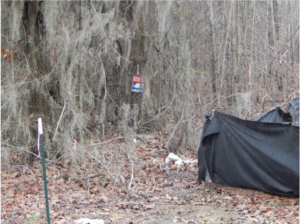
Improper Rain Gauge Placement 12.23.2013
